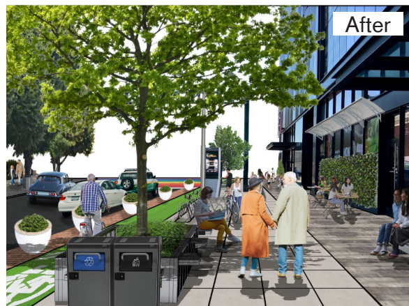
Enhancing walkability through safety measures (bike lane), aesthetic upgrades (tree pit, foliage), increased comfort (seating, awning), improved wayfinding, and energy-generating pavement.
